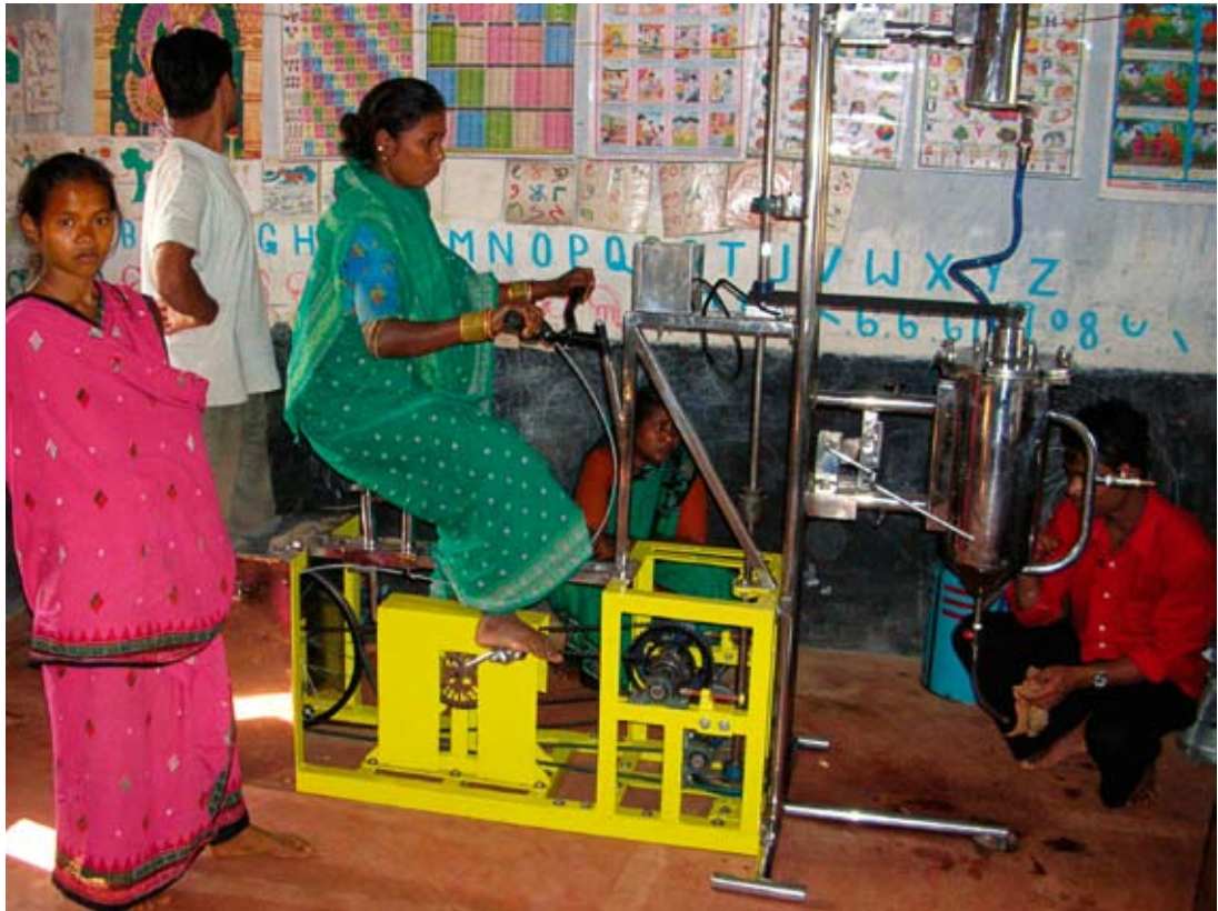
Photo: Pedal-driven Biodiesel Reactor; CT x GreEn
