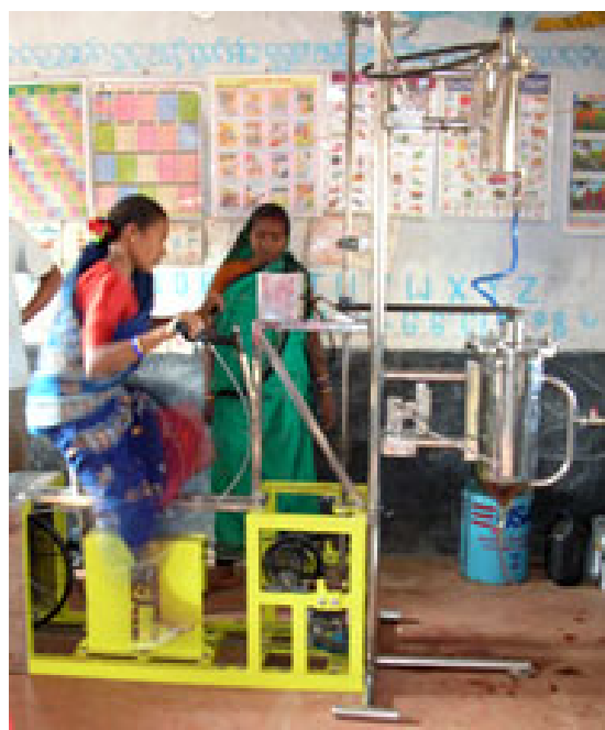
Figure 1. Pedal-powered Biodiesel reactor (capacity: 5 litres per batch)
