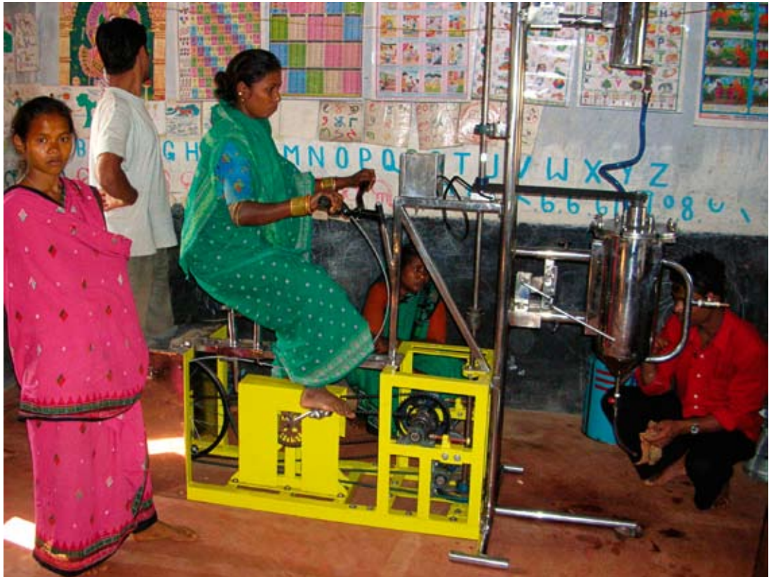
Photo: Pedal-driven Biodiesel Reactor; CT x GreEn
